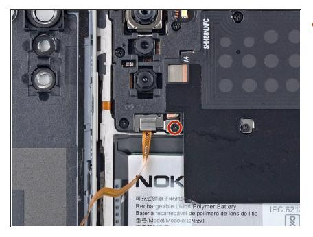
Use a Phillips screwdriver to remove the 3.8 mm-long screw securing the fingerprint reader bracket.
