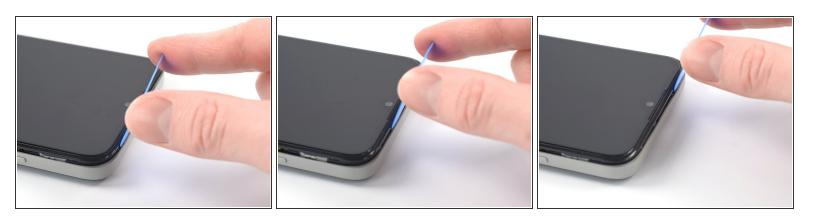
Slide the opening pick along the top edge of your phone to release the plastic clips.
