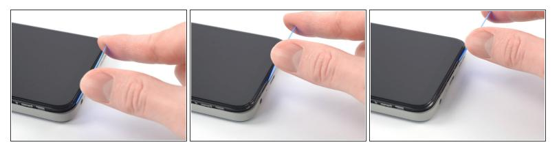
Slide the opening pick along the bottom edge of your phone to release the plastic clips.
