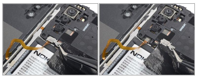
Use a pair of tweezers to remove the fingerprint reader bracket.
