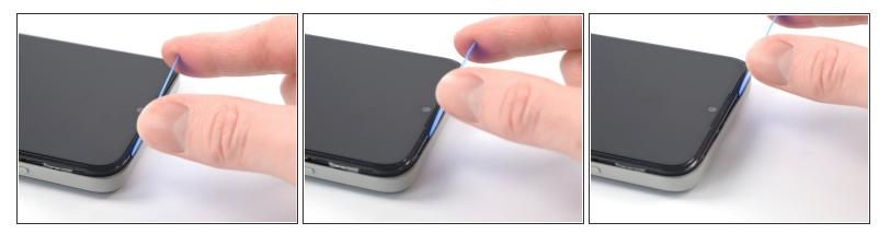
• Slide the opening pick along the top edge of your phone to release the plastic clips.
