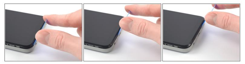
• Slide the opening pick along the bottom edge of your phone to release the plastic clips.
