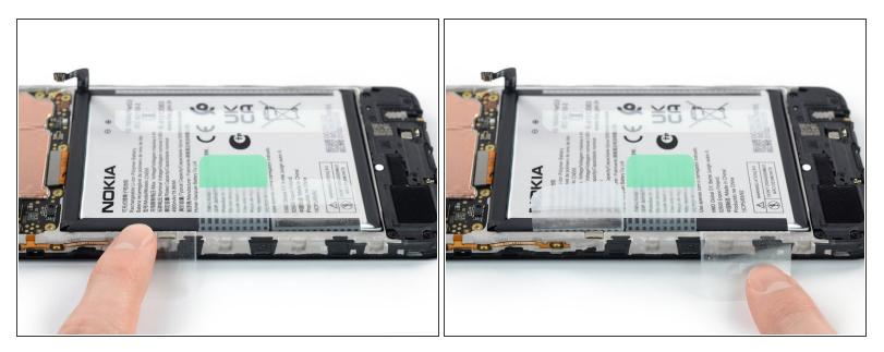
A Take care not to bend or puncture the battery during the next steps—a punctured or bent battery may leak dangerous chemicals or cause a fire.
